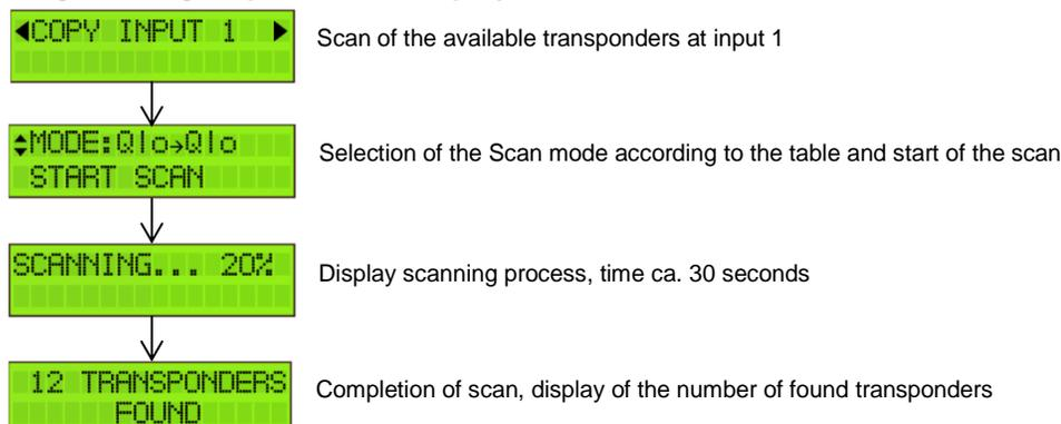
If it is necessary to change the transponders found, this can be done in the menu “**Input SAT 1-4**” via the item “**INPUT SAT 1**”. The transponders from the scan are displayed here.
