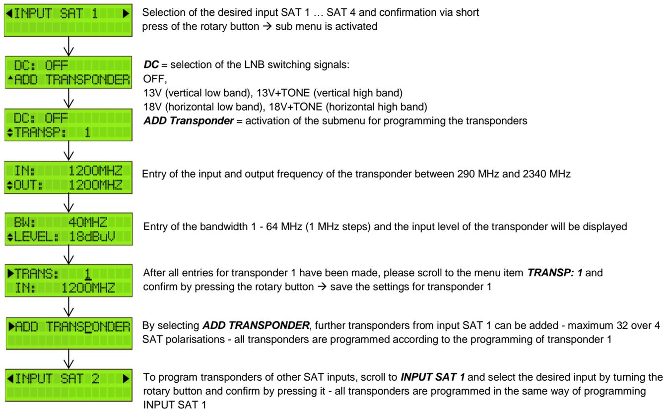
If it is necessary to delete a programmed transponder, this can be done by selecting the relevant transponder "TRANSP: 17" and pressing the rotary button for 3 seconds.
