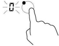
8. Touch timer control , The minder indicator will start flashing and "10" will show in the timer display.
