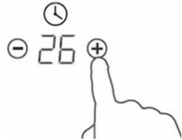
11. When the time is set, it will begin to count down immediately. The display will show the remaining time and the timer indicator flash for 3 seconds.
