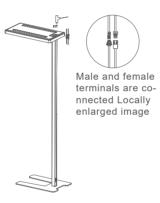
5.Install the top cover of the lamp cap; Finally, use 2 screws to lock the top cover of the lamp.
