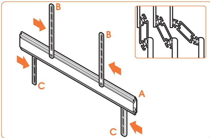
**3 If necessary, tilt the bar (A) in the desired position (see step 1).
