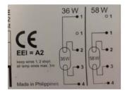
Step 2: Connect second fuse line to line "1"
