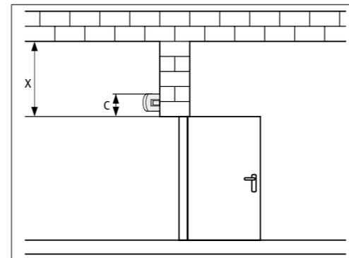
Swing door up to 3 m clear width, ceiling height above lower edge of lintel X up to 1 m (C = max. 0.1 m, X = max. 1 m)
