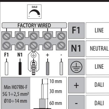
7C MIMIK 50 B DOUBLE SWITCH ON/OFF WIRING
