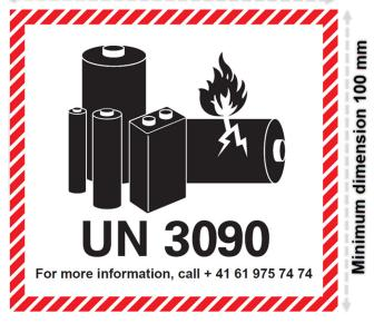
In case that the cell or battery is packed with or build-in equipment the UN Nr. must be amended to UN3091
