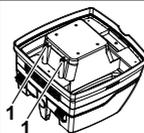
Clean the water level sensors (1) regularly and examine for signs of damage.
