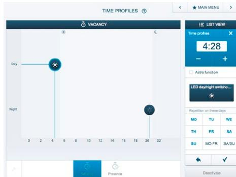
If you wish to control the device based on time, you can adapt the respective time profiles to your requirements. This specifies at which time of the day and date the devices are to be switched.
