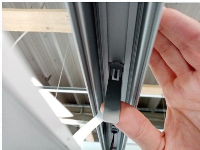
*Bend sheet metal lug 90 degrees upwards to secure it in place*
