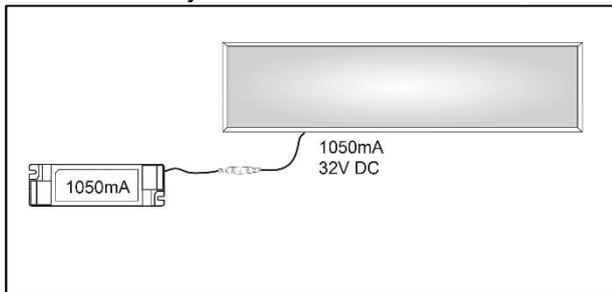
\*Do not connect the luminaire to an active LED driver. Some LED drivers emit high voltage when idle, which may cause permanent damage to the luminaire. Be sure to disconnect the LED driver from the power line before connecting the luminaire.
