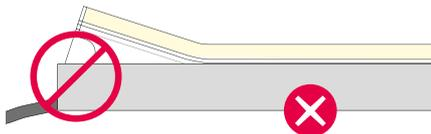
It is forbidden to force the **ST, SL, SR, SU** feed and the **end cap** of a welded feed into the profile and thus deform the LED strip light.
