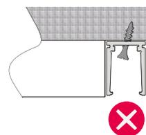
Gradient installing of screw.
