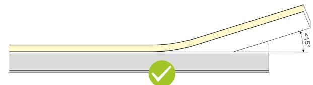
The installation angle must be **less** than 15° while the LED strip is pressed into the profile by hand to prevent damage to the circuit board.
