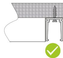
Install the screw into position and ensure the screw head is flush or lower the base of aluminum profile.
