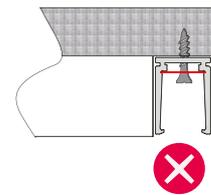
Screw head above to the base of aluminum profile.
