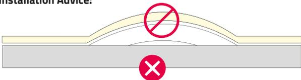
Install the light in **one** direction, no matter what kind of connector used. Don't let it choke in middle.
