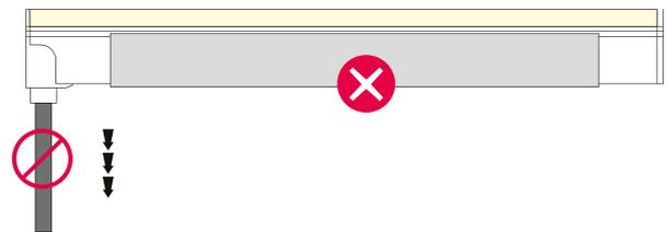
The supply cable must not be installed under any mechanical load (tension). It is forbidden to bend the cable with excessive force. It is recommended to lay the cable only after 60 mm in permissible installation radii.
