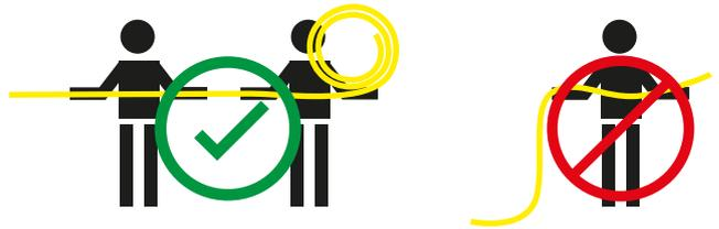
The LED strip must **not** be installed in a sagging manner. Installation by two people is recommended to **prevent** sagging.
