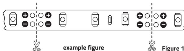
Separate the VARDAFLEX LED strip at the marked position. For a tightly assembled LED strip is a micro side cutter or an optional cutter required.
