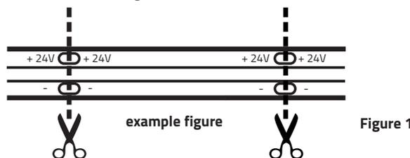
Separate the VARDIFLEX LED strip at the marked position. For a tightly assembled LED strip is a micro side cutter or an optional cutter required.
