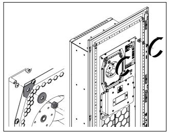
Fig. 13: Fit the top corner brackets
