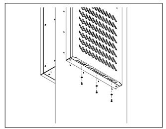
Fig. 39: Loosen the assembly screws
