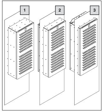
Fig. 8: Mounting options with a mounting frame
