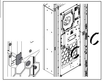
Fig. 16: Fit the central L-shaped brackets
