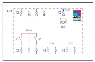
Fig. 29: Circuit diagram SK 3185.330
