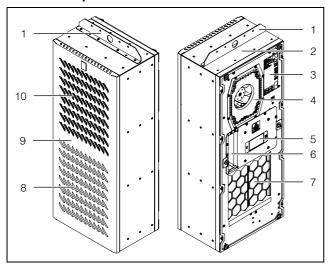
Fig. 2: Main components of cooling unit
