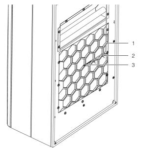
Fig. 35: Temperature sensor in front of cold air outlet (example illustration)
