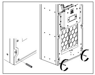
Fig. 10: Tighten the threaded bolts at the bottom
