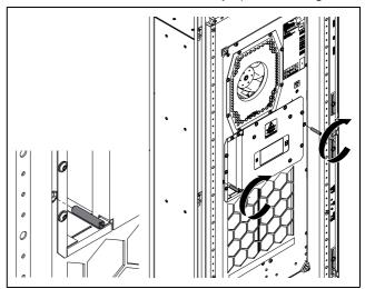
Fig. 15: Tighten the central threaded bolts
