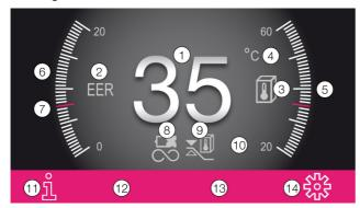
Fig. 33: Layout of the start screen
