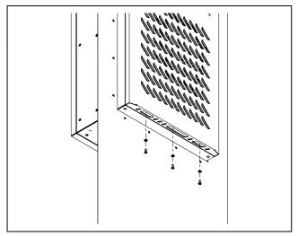
Fig. 22: Loosen the assembly screws
