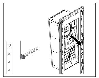
Fig. 12: Lower the cooling unit into the mounting cut-out
