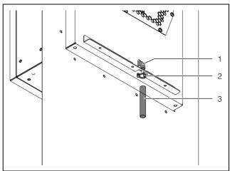
Fig. 25: Connection for condensate discharge hose
