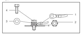
Fig. 28: Potential equalisation arrangement
