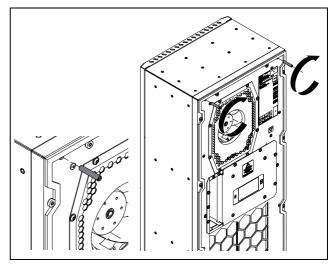
Fig. 11: Tighten the threaded bolts at the top
