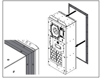
Fig. 18: Position the mounting frame
