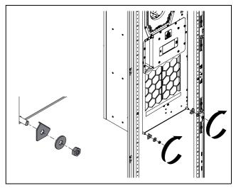
Fig. 14: Fit the bottom corner brackets
