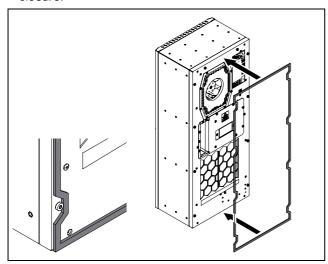
Fig. 9: Laying the seal
