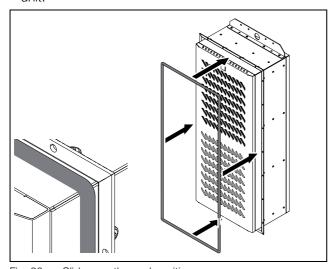
Fig. 20: Slide over the seal position
