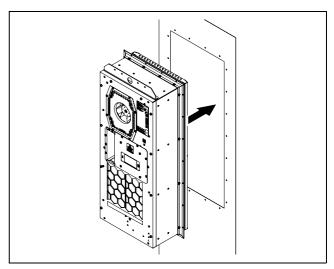
Fig. 21: Insert the cooling unit
