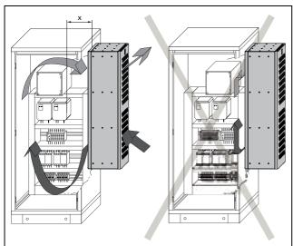
Fig. 5: Never direct the cold airflow at active components (example illustration)
