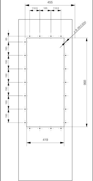
Fig. 43: Mounting cut-out
