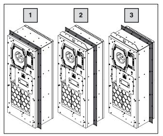
Fig. 17: Possible positions of the mounting frame
