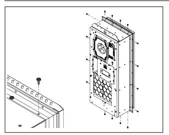
Fig. 19: Secure the mounting frame to the cooling unit
