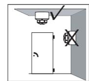
The Smoke Switch ORS 142 must be mounted on a horizontal surface as shown in the illustration. It is recommended to maintain a distance of 0.5 m from any installation.
