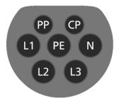
Figure 2: Assignment of the Type 2 connector for connection to the charging station (EVSE)
