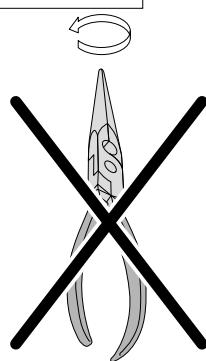
**EN** Rotation in counter-clockwise direction will destroy the adapter and its built-in electronic components.
