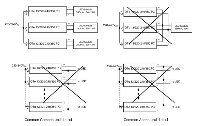
The installation of two or more OPTOTRONIC<sup>®</sup> OTe 13/220-240/350 PC Power Supplies with common "-" or "+" wiring by the intention to save wire to LED modules is prohibited, in order to avoid exceeding the maximum allowed system touch current levels on the accessible parts of the installation.
