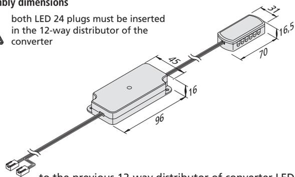
to the previous 12-way distributor of converter LED 24/...W
