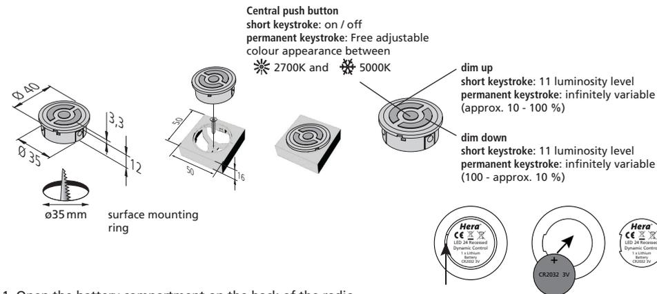
1. Open the battery compartment on the back of the radio telecontrol and insert the enclosed Lithium Battery CR2032 3V.
