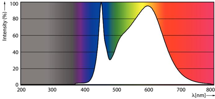
Spectral Power Distribution Colour - CorePro LEDtube 600mm HO 8W 840 T8
