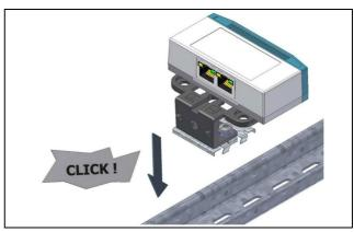
Fig. 6: Fastening the spring clip to the top-hat rail
